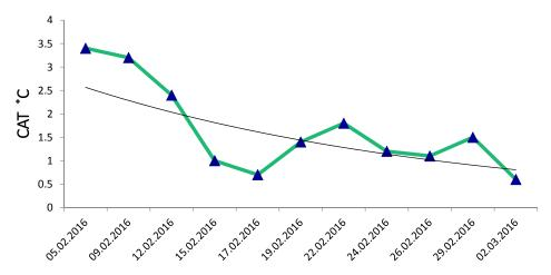
The variations in the CAT readings are expected to result from a combination of load fluctuations along with times when the condenser water strainer was becoming partially blocked. Accurate CAT results are taken when chillers are fully loaded. The Chiller 4 results provide the best indication of improvement.
